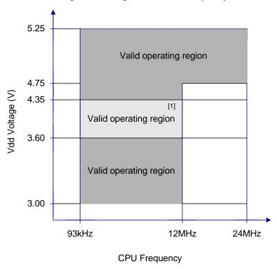
Figure 5. Voltage versus CPU Frequency
